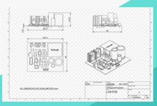
Interface PCBs for converting the voltage signals from the soil moisture sensors to 4-20mA current signals were fabricated
