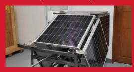
The entire solar panel deployment mechanism was also changed; in the prototype, easel-like panel stands had to be manually unfolded one by one by the user. On the contrary, this version employs two hand-operated winches and pulley mechanisms to easily unfold and fold the panels.
